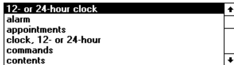
Figure 4-4. Use a list to reflect choices when those items vary as the application runs or when users are able to edit the items as they appear on the list.
