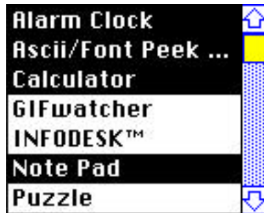
Figure 4-15. Use a list to present choices when those items vary as the application runs or when users are able to edit the labels of items as they appear on the list.
