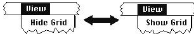
Figure 4-7. Shows the use of a toggled-menu item. Depending on the current condition (i.e., whether the grid is currently displayed or not) the menu item would change to reflect the command indicating the opposite action.
